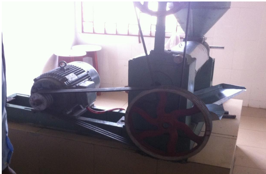
Moringa seed crusher used for the extraction of moringa oil.
